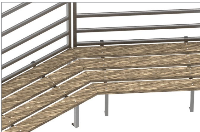
7 - Butt the second set up to first and fix in place.
