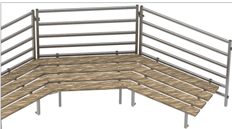
9 - Continue around the sections in this fashion until complete. When finished the brackets should be Dynabolted down.
