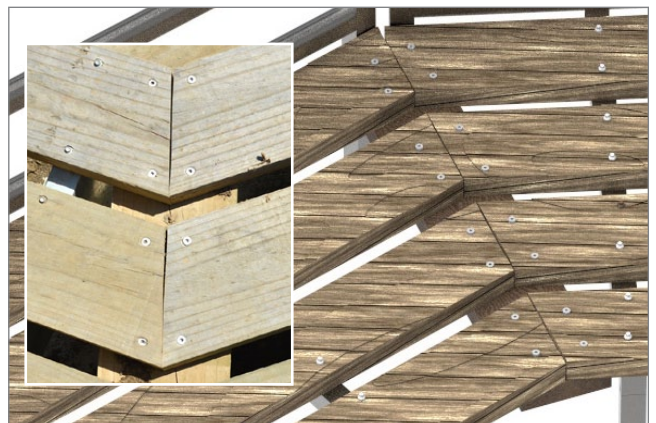
8 - Fix a plank beneath the unsupported ends to hold them in alignment and prevent trip hazard.
