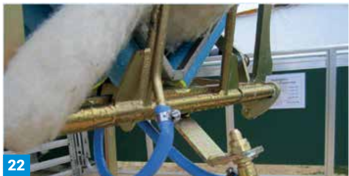
View of double spray system for rubber rings.
