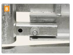
The yoke top adjustment A is made by a pin sitting through pre-drilled positioning holes. To adjust it, pull out the pin, move the yoke to desired position, then re-insert the pin through the positioning holes.
