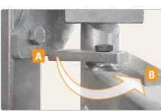
The Auto head bail' inward opening settings can be either narrowed to suit polled or dehorned cattle or widened to suit horned animals. Adjustment is made using the fitted gate stop lugs.
