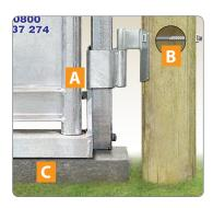
You should always mount the gudgeon pin plates with the top pin pointing up and the lower pin pointing down as this prevents animals from lifting the head bail.
