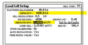
Press the blue soft key below CELL on the screen to enter the Load Cell Setup screen
