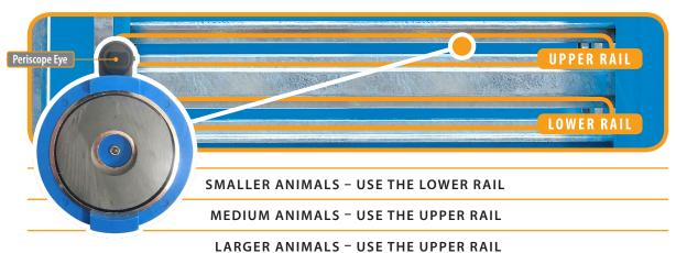
Please Note: The speed of the animals entering the DR3 will also affect the required eye position. Wool, dust and debris covering any of the eyes can affect their operation. Make sure that the lenses of the eyes are clear at all times.
