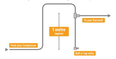
Pipe the air from the compressor to the Racewell via standard a 15mm (1/2 inch) alkathene water line. We have some Racewells working with the compressor up to 2kms away from the work site.
