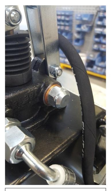
Photo 1 shows a large nut, remove this by turning anti clockwise.
