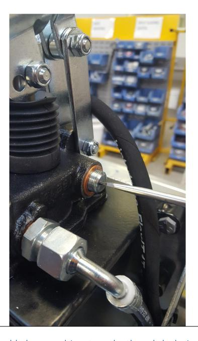
Using a large blade screwdriver turn the thread clockwise to increase the pump output pressure. Screw in one full turn and then try the pump. Repeat until pump has enough pressure to lift trailer off the ground.
