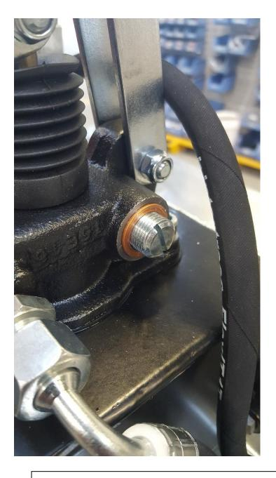
Once nut is removed a large thread will be revealed with a flat screwdriver head on it.
