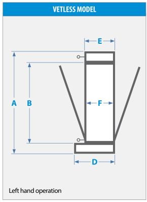
**Note:** These diagrams show left hand operation and our standard hinging configuration. Both side gates are hinged at the rear of the crush and open at the front. Right hand operation is a mirror image of the diagrams.
